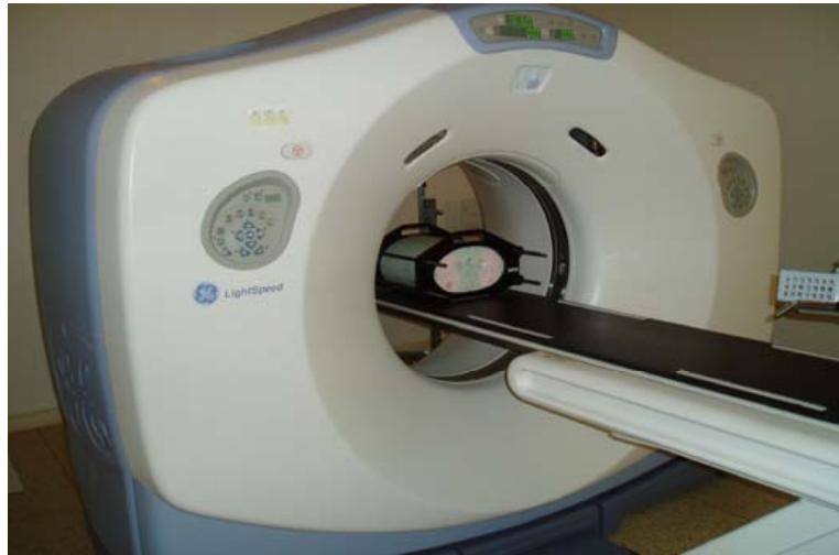
Figure A.2. Set-up of CIRS 002LFC phantom during CT scanning.
